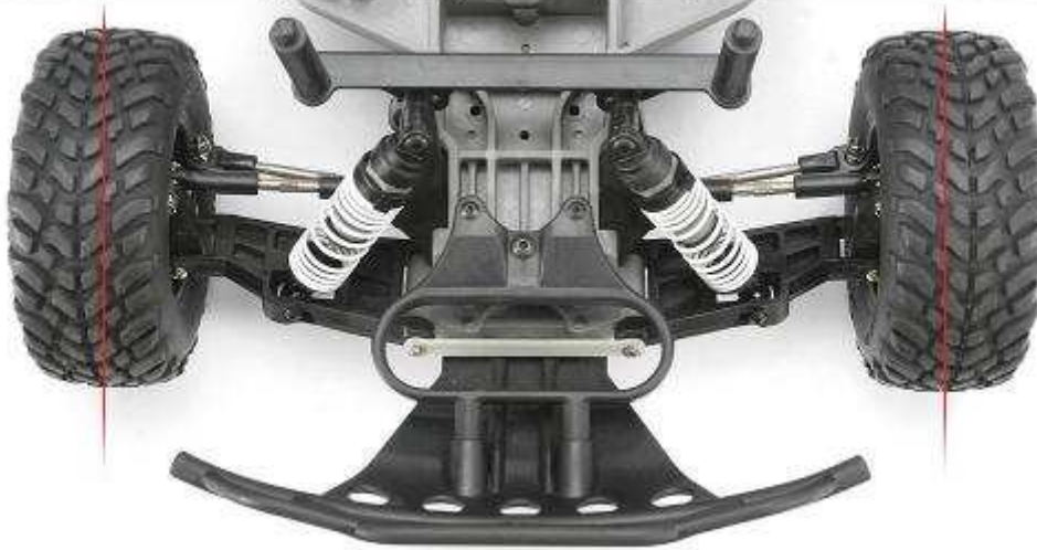
0-Degree Toe Angle – wheels straight forward
